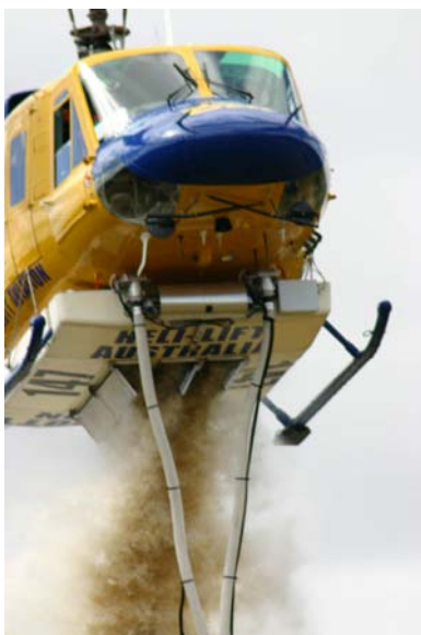
Belly tank testing of Helitack 147
