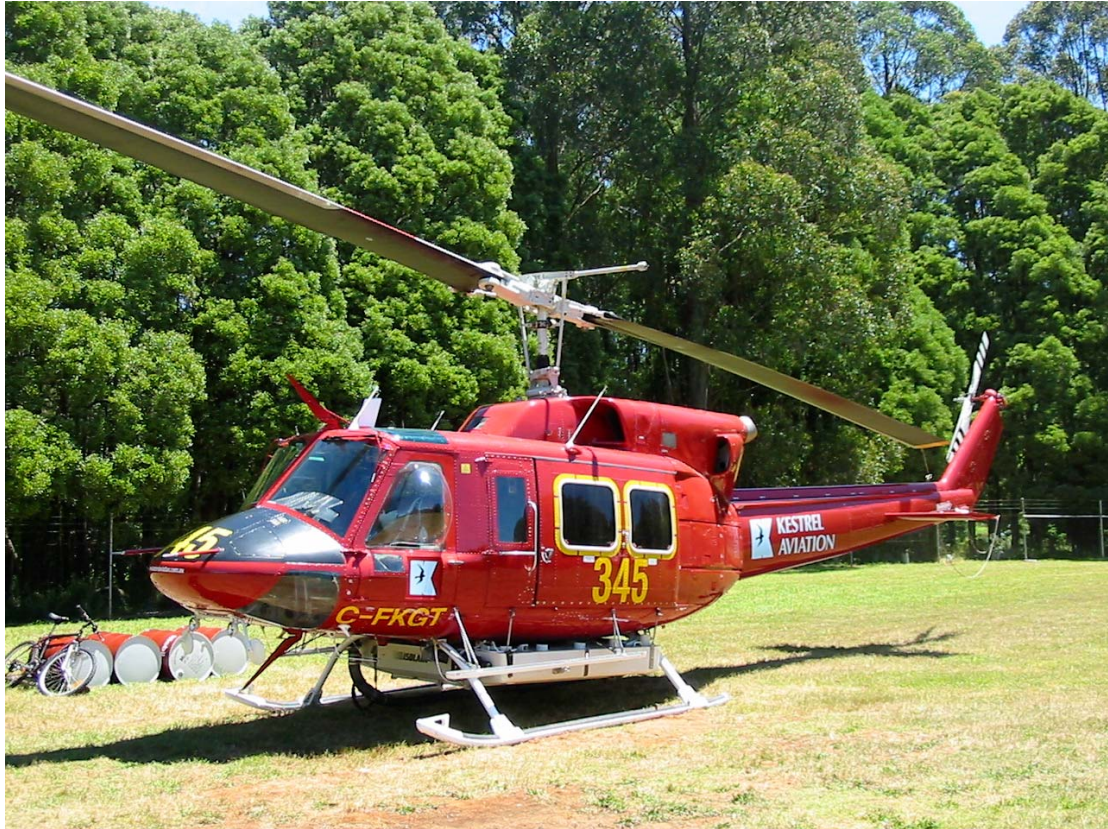
Helitack 345, a Bell 212 Type 2 firebombing helicopter, based at Olinda.
